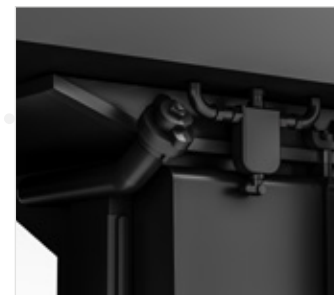
Separately fitted fuel filler neck
