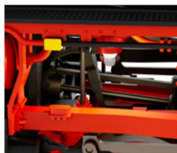
Replica of the third inside cylinder
