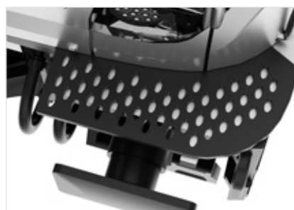
Shunting steps produced as openwork etched parts
