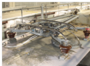
DSA 200 pantograph with concealed mounting
