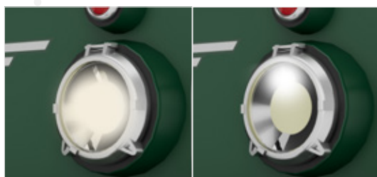
Headlights with low-beam and parking light functions
