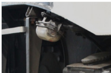
BR 139 with digitally controlled approach lights in the undercarriage area
