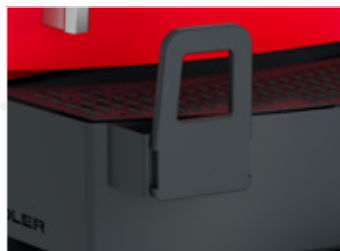
Freestanding shunting handles on the buffer beam
