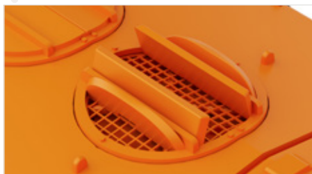
Fan cover in the open position, with the etched grille shown underneath
