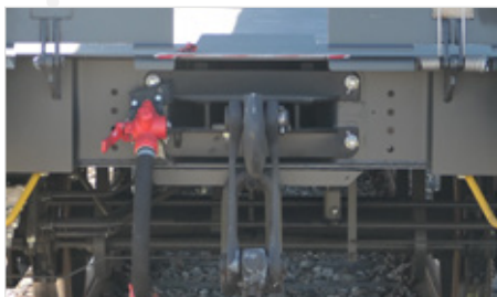
Buffer beam can be fully equipped with brake hose and coupling replica
