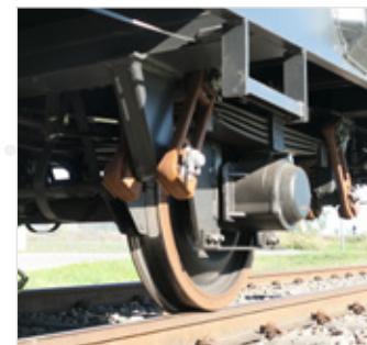
Multi-part design around the axleboxes and wheelsets
