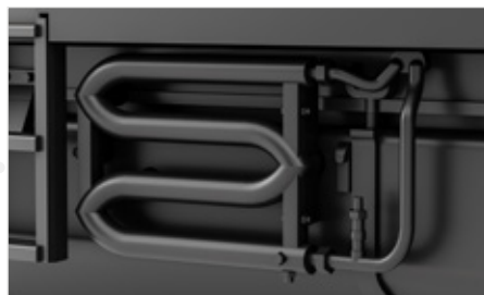
Freestanding cooling coils on the tank
