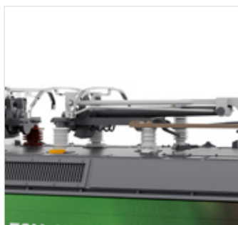
Current collector with no visible fixings
