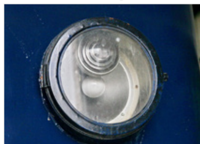
Headlamps with dipped-beam and parking light functions, faithfully reproduced in their original design
